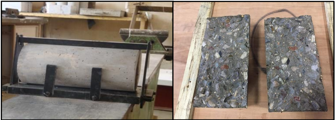
Figure (5) Splitting tensile strength test
