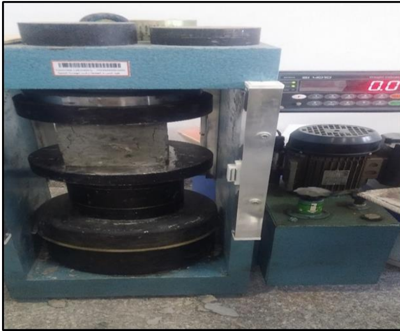
Figure (3): Compressive strength test of concrete
