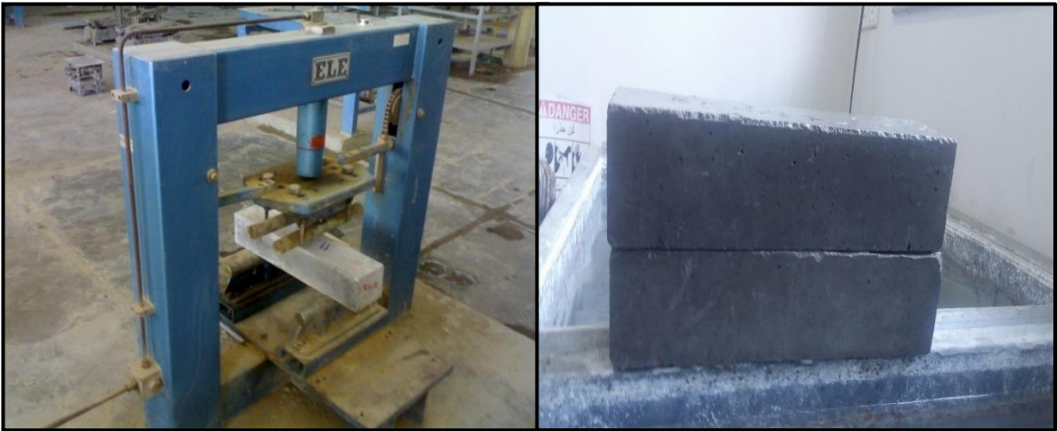
Figure (7) Modulus of rupture test
