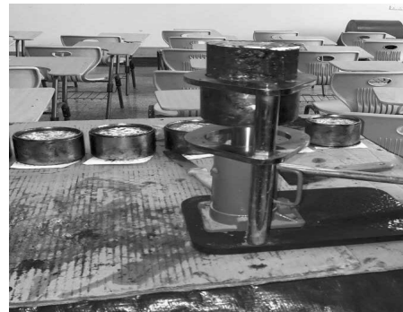
e: Extraction of Specimens from the Mold Using Mechanical Jack.
