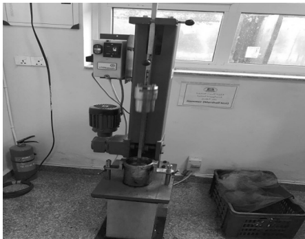
d: Compaction of Specimens.
