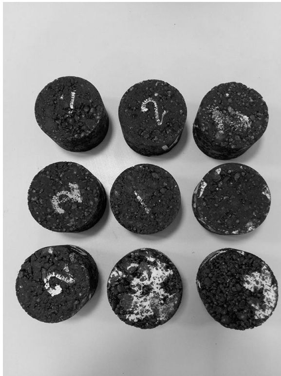
g: Marshall Specimens According to Optimum Asphalt Content.
