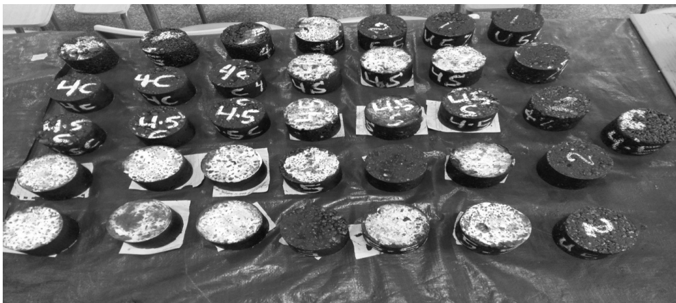
f: Marshall Specimens after Extraction from Molds.
