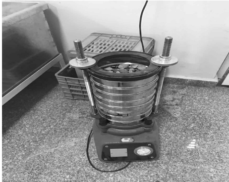
a: Sieve Analysis of Aggregate.
