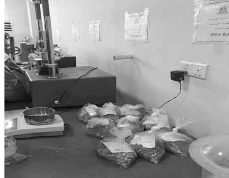
b: Preparation of Aggregate Sample.
